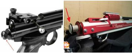
**Allowed**: Rear-mounted Velocity Adjuster **Reasoning**: The Adjuster is an integral part of the gun, and in some cases an after-market upgrade. It does not provide additional support.
